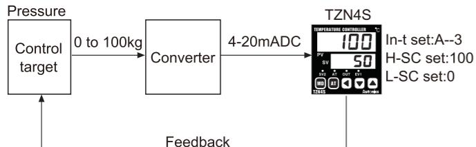
\* In case of using the converter mode, please select the inner switching pin according to the chart in "Selection switch for Input sensor/Voltage/Current".
