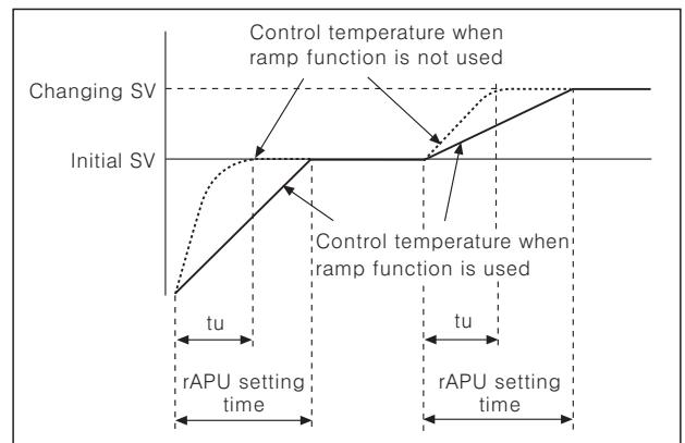
It makes delay rising temperature when change the set value at stable control status or delay the initial rising temperature as like above picture.
