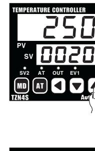
④ Press **MD** key when the setting is completed. It will stop flickering, then return to RUN mode.
