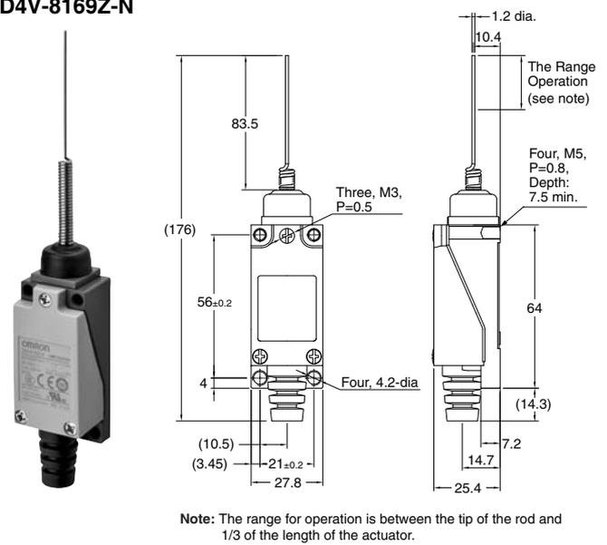
**Note:** Unless otherwise specified, the tolerances are  $\pm 0.4$  mm for the above dimensions for each model.
