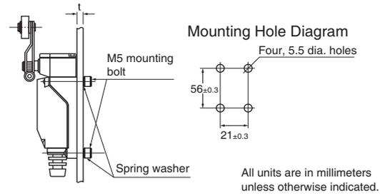
**Note:** The tap screws for the body are M5, P=0.8, with a minimum depth of 7.5 mm. Use bolts with a length of the panel thickness  $t + 7$  mm or less.
