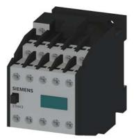
Contactor relay, 55E, EN 50011, 5 NO + 5 NC, screw terminal, AC operation, 230 V AC 50/60 Hz
