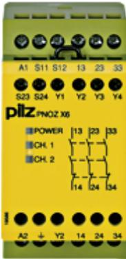
Safety relay (standalone) Inputs: 1-/2-channel wiring without detection of shorts across contacts Outputs: 3 N/O. Automatic/monitored start UB 230 - 240 V AC, width: 45 mm, plug-in terminals of screw type Monitoring E-STOP, safety gates.
