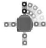
The SLK can be operated both horizontally and vertically. The necessary pre-setting is carried out before mounting by simply adjusting the actuating head. This flexible method of mounting is supported by the ability to position the actuating head in 4 x 90° increments.
