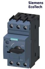
Circuit breaker size S00 for motor protection, CLASS 10 A-release 10...16 A N-release 208 A screw terminal Standard switching capacity
