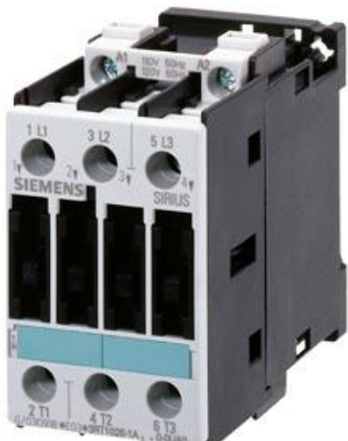
CONTACTOR, AC-3 11 KW/400 V, DC 220 V, 3-POLE, SIZE S0, SCREW CONNECTION
