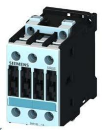
CONTACTOR, AC-3 5,5 KW/400 V, AC 230 V, 50/60 HZ, 3-POLE, SIZE S0, SCREW CONNECTION  $\,$
