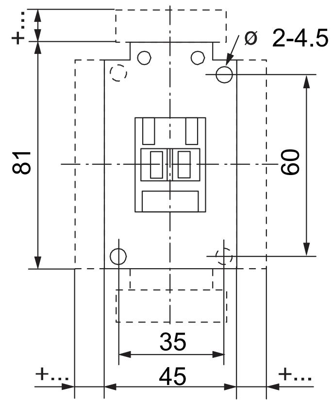
Allen-Bradley 100C Contactor 4kW 3Pole 24VAC 50 and 60Hz Coil 1NO Contact Auxiliary
